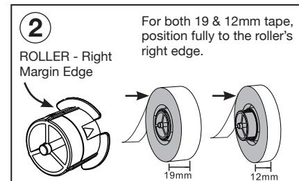
For both 19 & 12mm tape, position fully to the roller's right edge.
