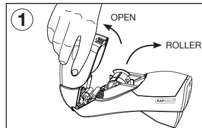
Press "OPEN" at the rear of the transparent cover and take out the roller.
